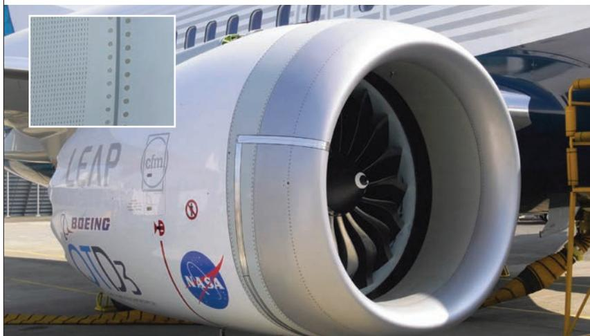
**Silver tape covers wiring to a noise sensor in the inlet (inset) which was configured with the new low-drag slotted face sheet.**
